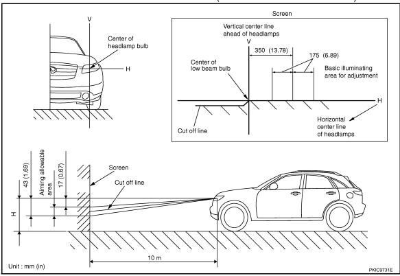
If the vehicle front body has been repaired and/or headlamp assembly has been replaced, check aiming. Use the aiming chart shown in the figure.
