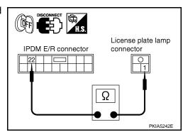
6. Check continuity between IPDM E/R harness connector and rear combination lamp harness connector.
