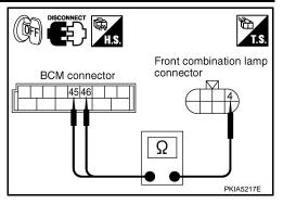
4. Check continuity between BCM harness connector (A) and side turn signal lamp (RH and LH) harness connectors (B).
