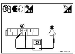
5. Check continuity between BCM harness connector (A) and rear combination lamp (RH and LH) harness connectors (B).
