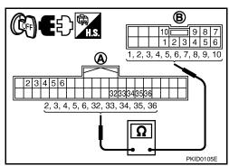
Check for continuity between each of BCM harness connector in suspect malfunctioning system and ground.
