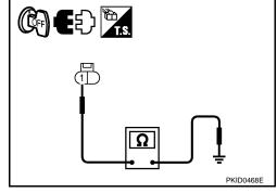
3. Check continuity between rear combination lamp (RH and LH) harness connectors and ground.
