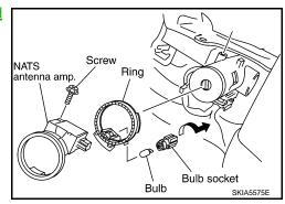
IGNITION KEY HOLE ILLUMINATION (with Intelligent Key)
